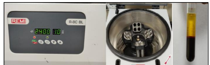
Fig 5: Centrifuge first spin: 2400RPM x10 minutes
